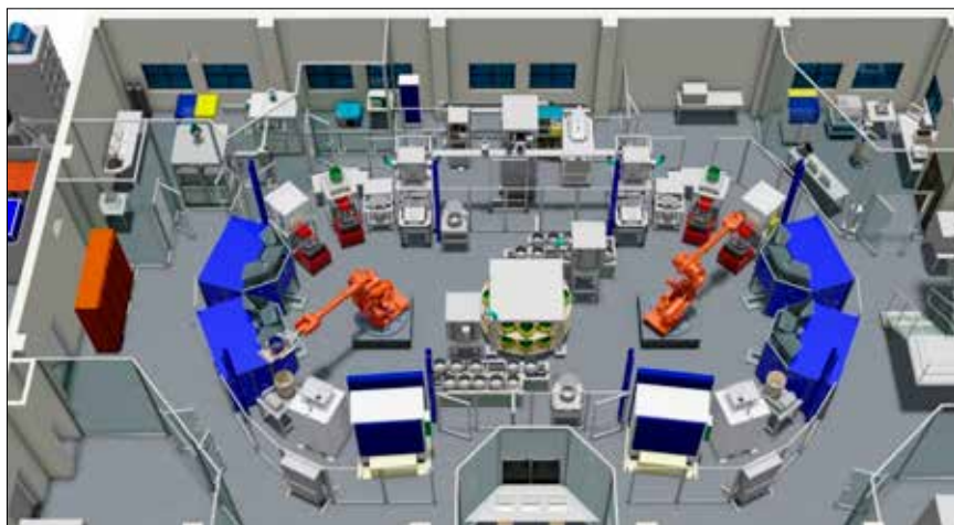
Figure 1. Robotic automation for sampler preparation and analysis for chemical, PSD and moisture conveyor.
