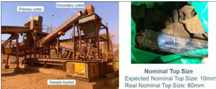
Figure 1. Quantified field evidence (right) collected after a visual inspection of the primary sample station shown on the left. The deviation between the expected nominal top particle (10 mm) and the factually observed size is dramatic.
