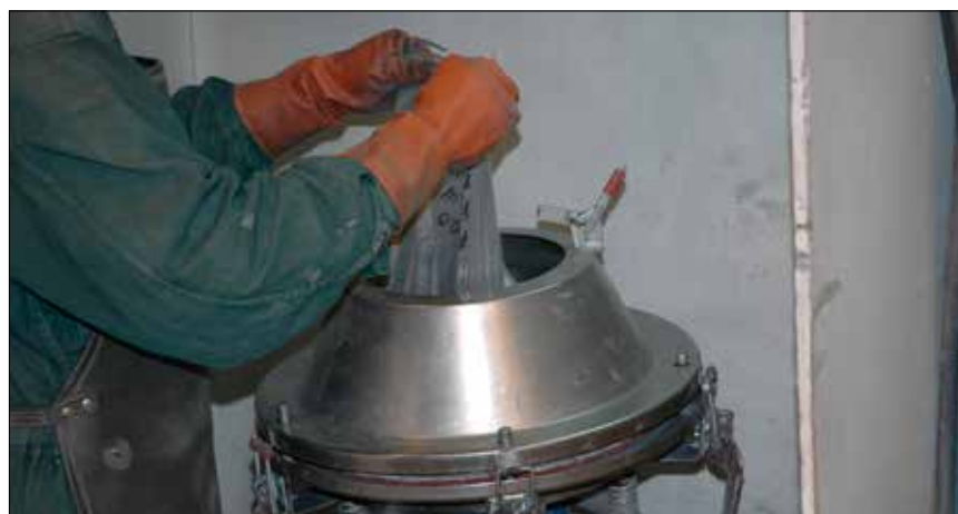
Figure 1. Screen fire assay is always a good option in the presence, or suspected presence, of coarse gold. It provides a good spatial measure of the problem. It is important to ensure that a nylon screen is used that is fire assayed to extinction. This removes sample-to-sample contamination of the screen. Duplicate or triplicate fire assays should be applied on the undersize fraction to check the level of heterogeneity—some “fine” coarse gold can still pervade the fine fraction.
